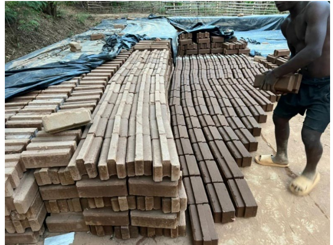
A worker making bricks - Clay resourced on site is used for brick production, reducing the environmental footprint.
